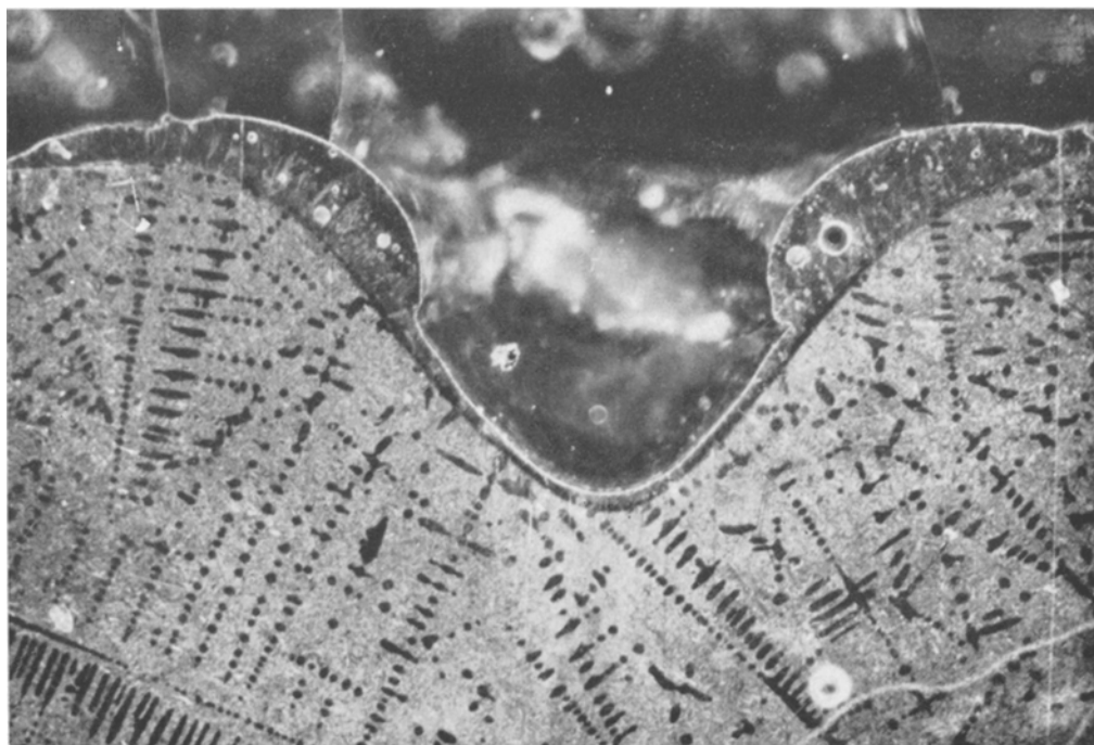
Figure 1 Section of a laser-irradiated silver-21 at. % germanium alloy. Unetched ( \times 60 ).
